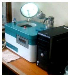
Fig. 4: Bomb calorimeter used to determine the calorific power.
