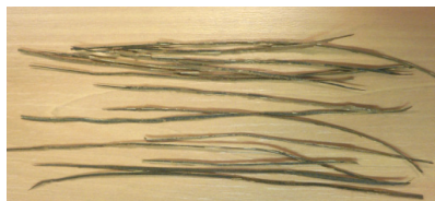
Fig. 1: Fibres of palmyra extracted for the tensile tests (Ngargueudedjim et al. 2016, Allarabeye 2010).
