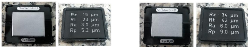
Fig. 7: Metal master pieces of the perthometer.
