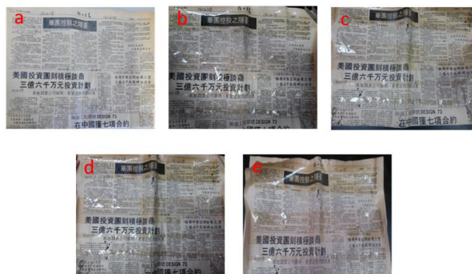
Fig. 1: The aging of PtBA adhesive coated on CDN. (a) Unaged; (b) Aged for 24 h; (c) Aged for 48 h; (d) Aged for 72 h; (e) Aged for 96 h.
