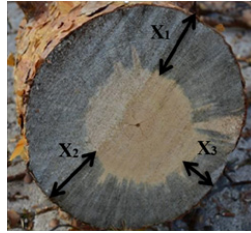
Fig. 1: Cross-section of the blue stained log and the measurement of degradation width (Komut and Ozturk 2018).
