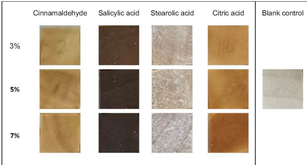
Fig. 3: The color of poplar specimens after impregnated with different compounds.
