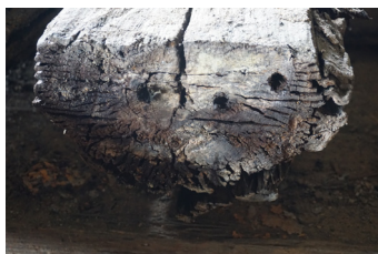
Fig. 1: Wooden board after extraction of samples in axial direction.
