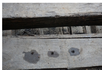
Fig. 2: Wooden board after extraction of samples in radial direction.
