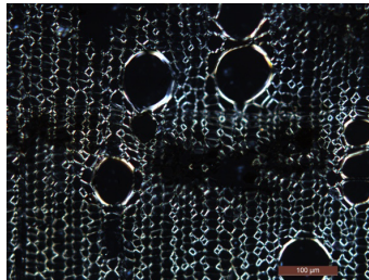
Fig. 6: 0.8 cm deep in axial direction, heartwood, under cross polarizer.
