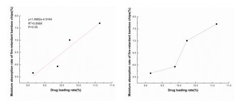
Fig. 5: Correlation analysis of drug loading Fig. 6: Effect of drug loading rate on water rate and water absorption rate of fire retardant absorption rate of fire retardant bamboo chips. bamboo chips.
