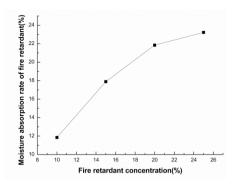
Fig. 1: Effect of fire retardant concentration on water absorption rate of fire retardant.
