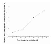
Fig. 2: Effect of fire retardant concentration on water absorption rate of fire retardant bamboo chips.
