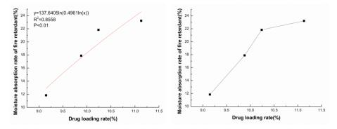
Fig. 3: Correlation analysis of drug loading rate and water absorption rate of fire retardant.
