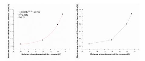
Fig. 7: Correlation analysis of water absorption rate on fire retardant and fire retardant bamboo chips.
