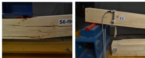
a) Bending failure.
