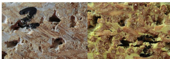
Fig. 1: Cross-sectional view of wood-wool panel before and after wet and dry treatment.
