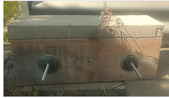
Fig. 1: Experimental sample of composite timber-concrete beam.
