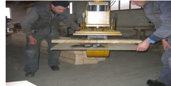
Fig. 6: The embedding of the connector plate into the wood.
