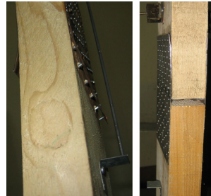
Fig. 14: Ratio between limit bearing capacities of connectors (%). Fig. 15: Deformation of connection.
