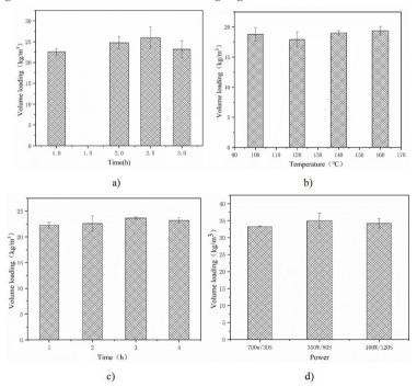
Fig. 2: Effect of pretreatment on the volume loading: a) NaOH pretreatment, b) heat treatment, c) ethanol extraction, d) microwave treatment.
