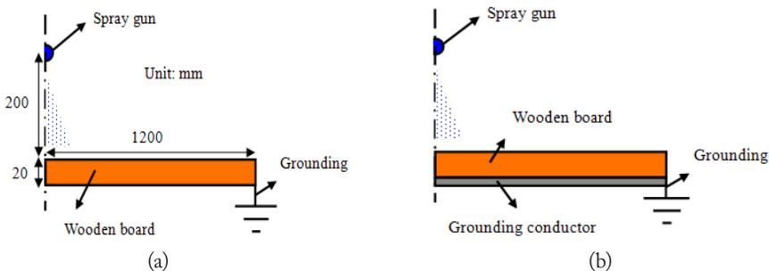
Fig. 4: Simulation models of two electrostatic spraying methods.
