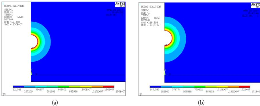
Fig. 8: Electric field intensity of two electrostatic spraying methods.
