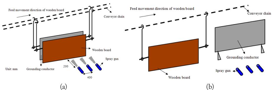
Fig 1: electrostatic spraying of wooden board with a grounding conductor. (a) way 1; (b) way 2.
