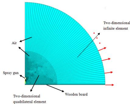
Fig. 5: Finite element model after meshing.
