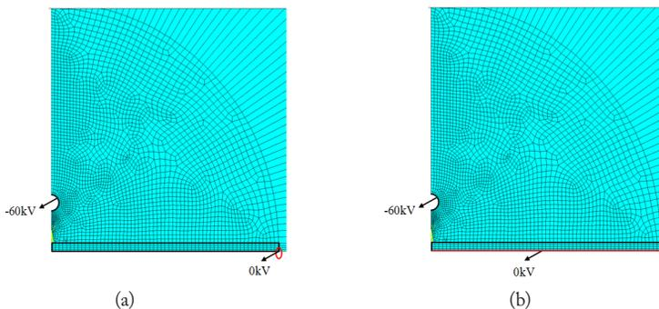
Fig. 6: Boundary conditions of two electrostatic spraying methods.
