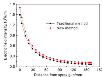
Fig. 9: Electric field intensity distribution under the electrostatic spray gun.
