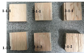
Fig. 9: Adhesive layer shear failure of CLT specimen.
