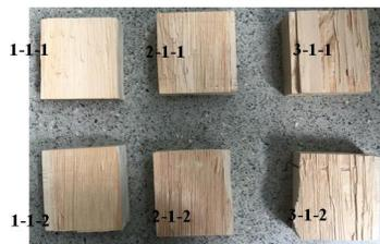
Fig. 9: Adhesive layer shear failure of CLT specimen.
