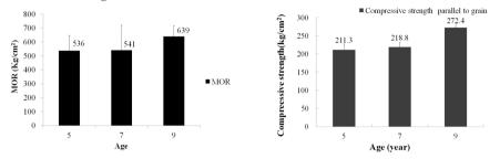
Fig. 4: Average modules of rupture (MOR) Fig. 5: Average compressive strength perpendicular of Paraserianthes falcataria wood from three to grain of Paraserianthes falcataria wood from different age of tree.
