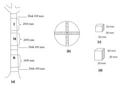
Fig. 1: Schematic drawing of preparing sample. (a) Log and disk cutting. (b) Transversally schematic diagram of preparing sample of moisture content, density, and shrinkage measurement. (c) Preparing sample for moisture content and density measurement. (d) Preparing sample for shrinkage measurement.
