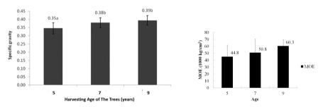
Fig. 2: The Average specific gravity of Paraserianthes Fig. 3: Average modules of elasticity (MoE) falcataria wood from three different rotation age of of Paraserianthes falcataria wood from three tree.
