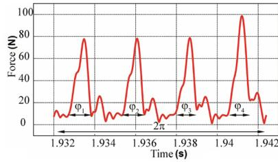
Fig. 3: Change of the main cutting force for one cutter revolution.
