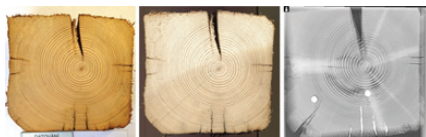
Fig. 1: Photograph, scan (with measurement path) and X-ray scan of the sample of Abies .
