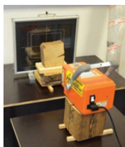
Fig. 5: X-ray scan device EcoRay HF 1040 and measuring of the sample.
