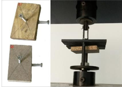
Fig. 1: Withdrawal resistance test, (1) BOSB; (2) CPB.
