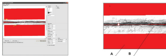
Fig. 8: Area quality in "Surface" software, software evaluation (left), areas ratio (right) (A – undamaged, B – damaged).
