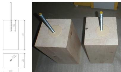
Fig. 1: Test sample geometry.
