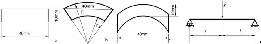
Fig.5: Schematic diagram of samples (a.b.c) and simplified mechanical model (d) a. rectangular bamboo; b. partial ring; c. arc bamboo.
