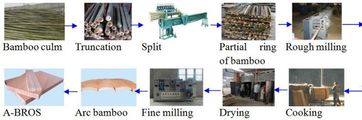
Fig.1: Process of arc bamboo manufacture in practice.
