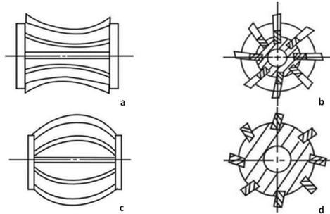
Fig.2: Schematic structure of upward (a b) and downward (c d) arc milling cutters.
