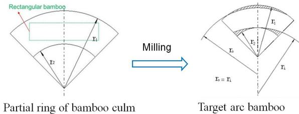
Fig.3: Schematic diagram of arc bamboo from partial ring of bamboo culm.
