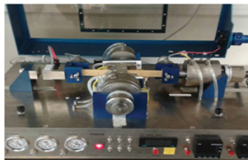
Fig. 1: Automated bond-evaluation system (ABES) used for the evaluation of bonding strength of veneers glued with PF adhesive.
