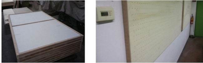
Fig. 1: Framed panels produced on the basis of impedance tube results: back of the panel filled with sound absorbing mats (left) and detail of a panel installed in end-use application (right).
