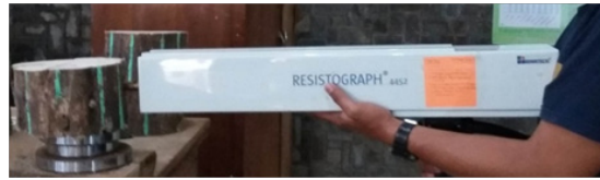
Fig. 1: Microdrilling resistance testing using Resistographâ.
