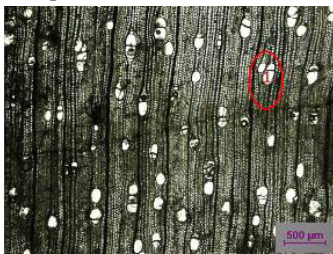
Fig. 9: The shape of vessels with rotundities and ovals in untreated alder birch wood sample (cross section, 4x).
