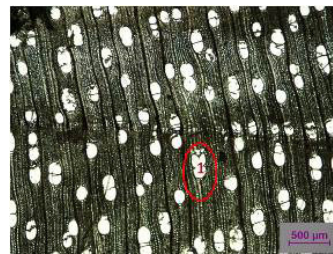
Fig. 10: Neither radial crack nor tangential crack, and neither collaps in the vessels nor in the fibres and ray cells was observed in heat-treated alder birch wood sample (cross section, 4x).
