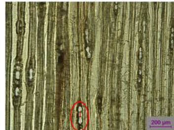
Fig. 6: Part of ray parenchyma cells, appeared to be damaged in heat-treated szemao pine wood sample (tangential section, 10x).
