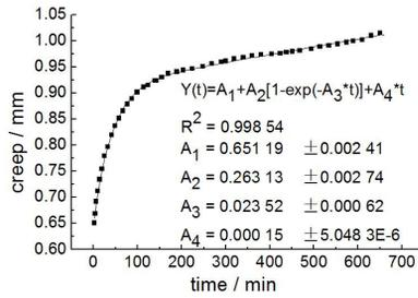
Fig. 5: Creep curve and fitting data of group MD. Fig. 6: Creep curve and fitting data of group MW.
