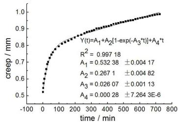
Fig. 4: Creep curve and fitting data of group LW.
