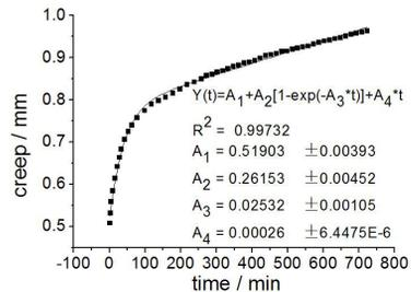
Fig. 9: Creep curve and fitting data of group LDP. Fig. 10: Creep curve and fitting data of group LWP.
