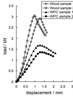
Fig. 2: Load-displacement curves of representative samples tested in screw holding power.
