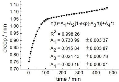
Fig. 7: Creep curve and fitting data of group HD. Fig. 8: Creep curve and fitting data of group HW.
