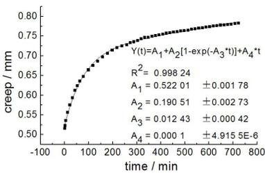
Fig. 3: Creep curve and fitting data of group LD.
