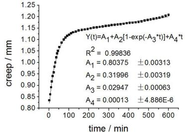
Fig. 11: Creep curve and fitting data of group MWP. Fig. 12: Creep curve and fitting data of group HWP.
