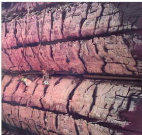
Fig. 5: Detail of the groove sealing disruption after 31 min of thermal loading.
