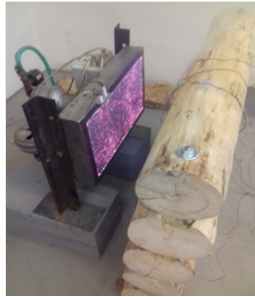
Fig. 4: Position of sample in front of the ceramic radiant panel.
