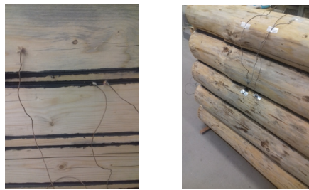
Fig. 3: Position of thermocouples located on the samples.
