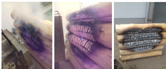
Fig. 7: Testing the Sample 1 a) after 10 min, b) after 30 min, c) after the testing.
