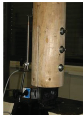
Fig. 10: The assessed joint with a slotted-in-steel plate and bolts. Fig. 11: The arrangement of the loading tests.
