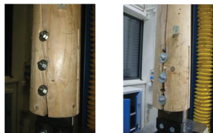
Fig. 12: Failure of tested samples (connections) after loading (on the left with strengthening on the right without strengthening).
