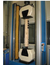
Fig. 10: The assessed joint with a slotted-in-steel plate and bolts. Fig. 11: The arrangement of the loading tests.
