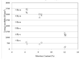
Fig. 1: Moisture dependent Young's modulus of face layers determined by ultrasound (u) and compression (c) tests.
