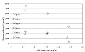
Fig. 4: Moisture dependent shear modulus of core layers determined by ultrasound (u) and compression (c) tests.
