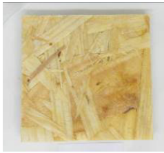
Fig. 3: Result of mould growth on oriented straight board (OSB) tested according to EN 14119, method A2.
