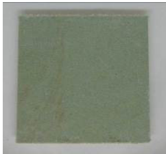
Fig. 5: Results of fungal growth of plasterboard (SDK) tested according to EN 14119, method A2.
