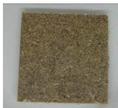
Fig. 1: Result of mould growth on particleboard tested according to EN 14119, method A2.
