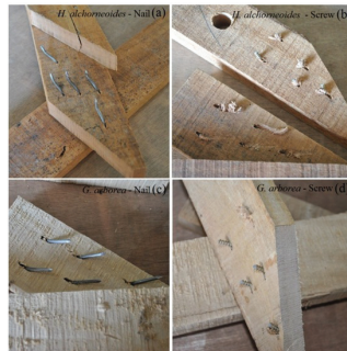
Fig.3: Types of fastener failure of nail and screws in H. alchorneoides joints at 30° (a and b, respectively) and G. arborea joints at 30° (c and d, respectively).
