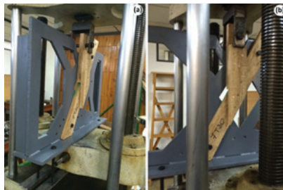
Fig.2: Test frame device employed for testing joints (a) and applying loads during tests(b).
