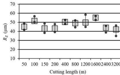
Fig. 2: Surface roughness  $R_z$  of birch test pieces across fibre planned with ET1.
