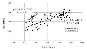
Fig. 2: Relationship between bending MOE and the density of wood in air-dry condition (moisture content of wood =12 %).
