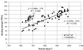
Fig. 3: Relationship between static bending strength and density of wood in air-dry condition.
