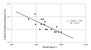
Fig. 5: Relationship between content of mineral substances and density.
