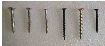
Fig.1: Screws used in this study (from left to right in the order of self-tapping screws (diameter of 6, 5 and 4 mm), chipboard screw, wood screw, and drywall screw).
