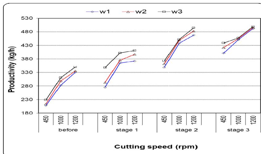
Fig. 4: The relationship between cutting drum speed and productivity at three levels of feeding capacity (w1, w2 and w3) for wood residues at 7.2% moisture content.
