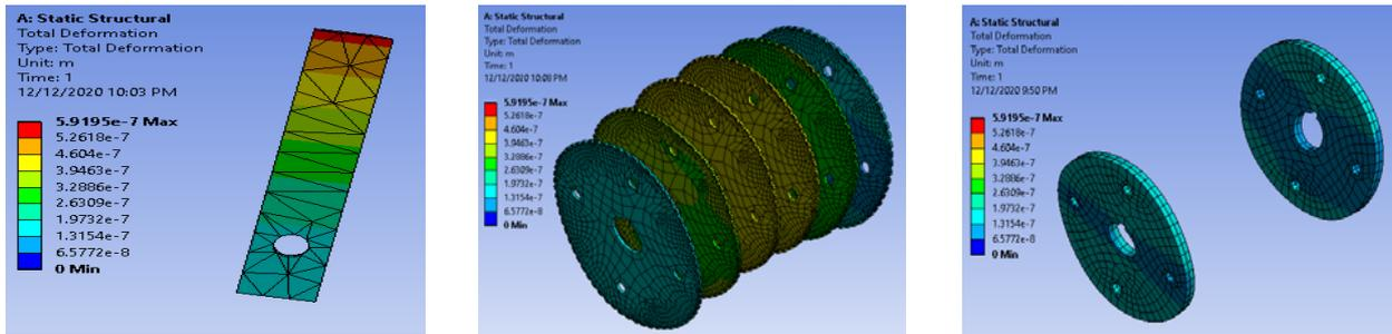
Fig. 2: Model analysis of the knife, disk and flange deformations in Ansys Pro.
