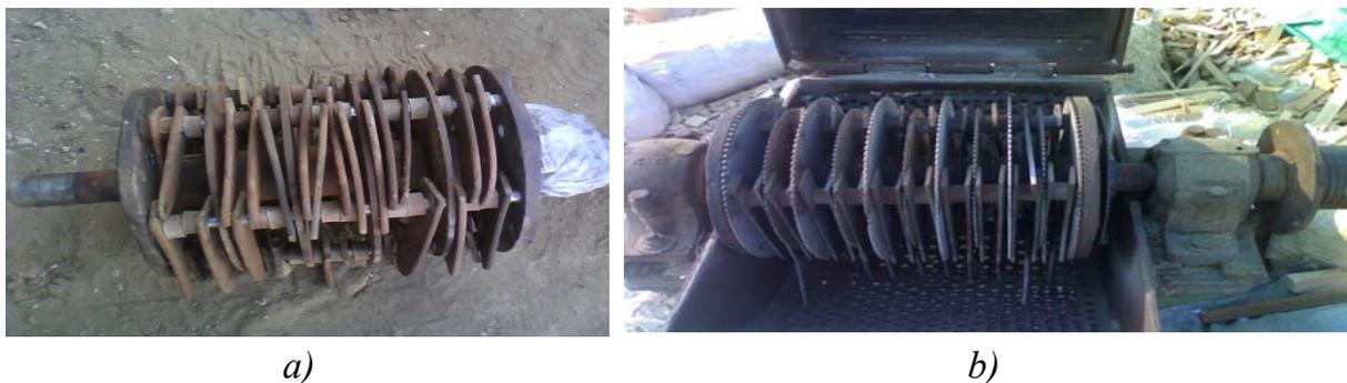
Fig. 1: a) The old drum under study before modification and b) after modification.
