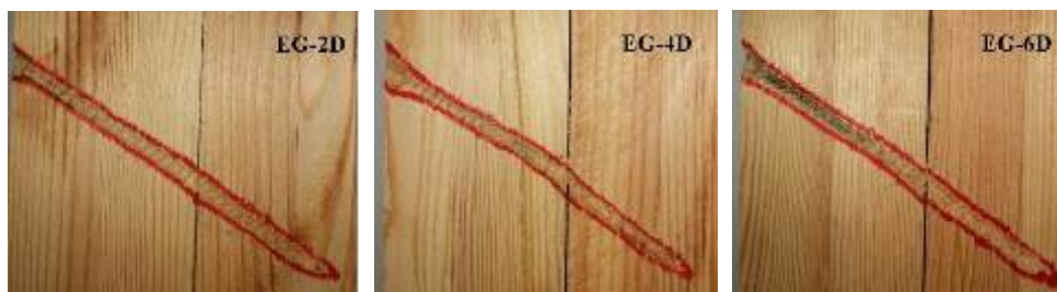
Fig. 15: Inside phenomena of specimens with different edge distances.
