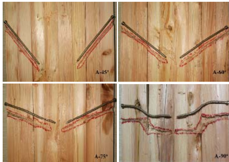
Fig. 11: Inside phenomena of different anchorage angles.
