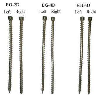
Fig. 16: The failure mode of the self-tapping screw.
