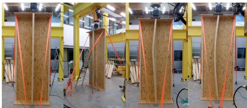
Fig. 2: Wall panel placed to the test area: axonometry and front view (on the left), deformed structure: buckling of the free flange of I-stud and deflection of the entire I-stud in the plane of the wall (on the right).
