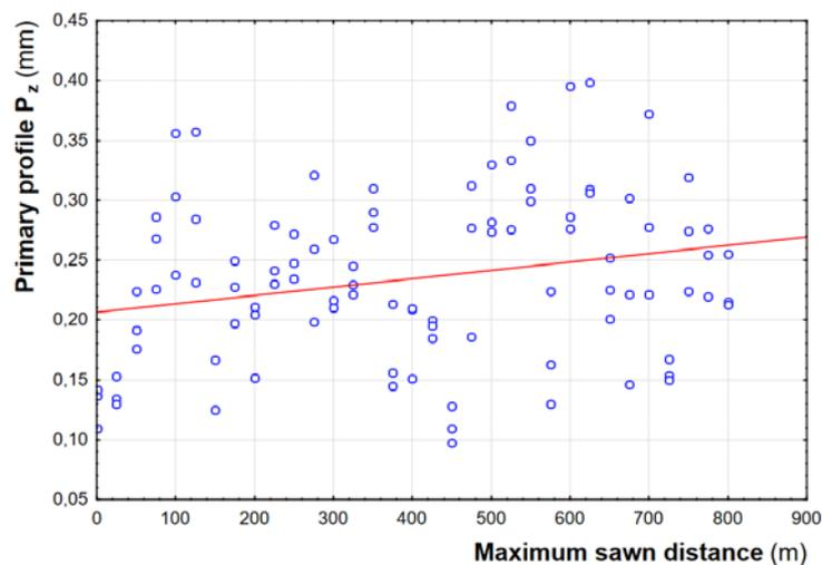
Fig. 12: Correlation of primary profile  $P_z$  and maximum sawn distance for saw blade 60T.
