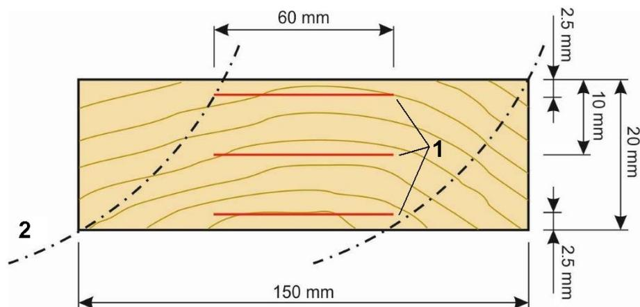
Fig. 6: The schematic representation of measuring locations on the transversal surface: (1) measuring paths; and (2) track teeth of the saw blade.
