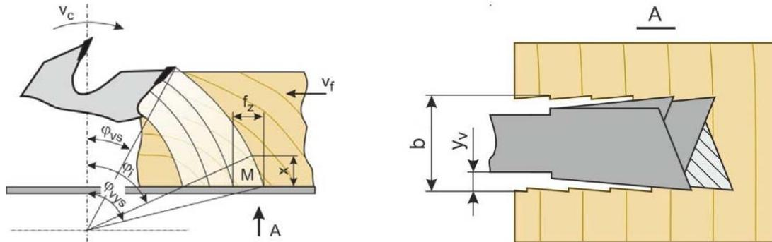
(Note:  $v_c$  - cutting speed,  $v_f$  - feed speed,  $f_z$  - feed per tooth,  $\phi_{vs}$  - feed angle of the cutting edge entry into the wood,  $\phi_{v's}$  - feed angle of the cutting edge exit from the wood,  $\phi_i$  - feed local angle corresponding to the monitored point M,  $b$  - cut gap width, and  $y_v$  - saw teeth setting) (Kminiak and Gaff 2015).
