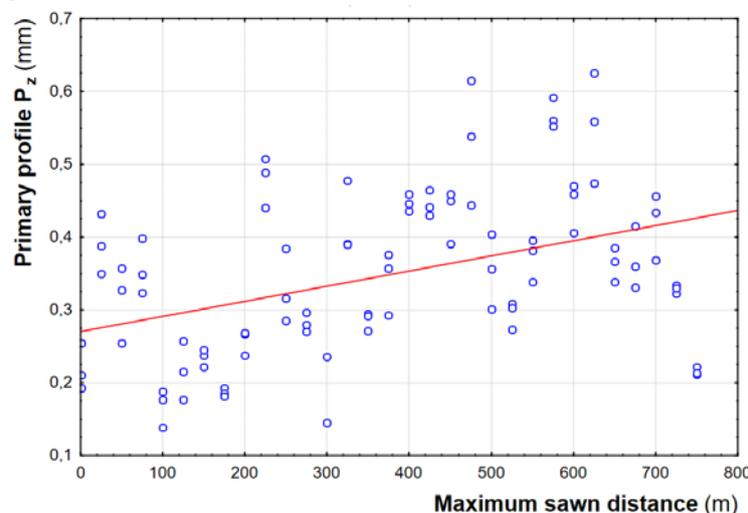
Fig. 10: Correlation of primary profile  $P_z$  and maximum sawn distance for saw blade 24T.
