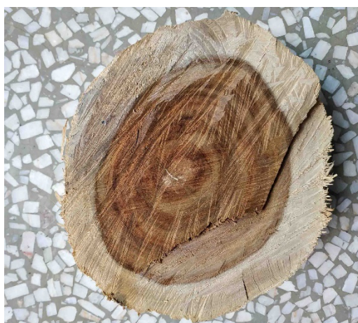
Fig. 1: A cross section of the base of a 15-year-old Dalbergia sissoo stem, indicating the difference in color between the heartwood and the sapwood of the wood.
