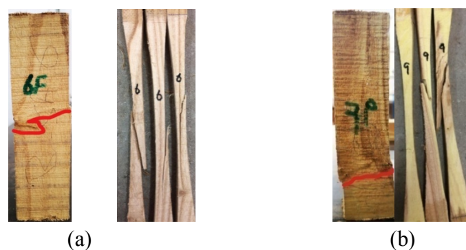
Fig. 5: Failure pattern under compression for Melia Azedarach (Dhariak) from city of (a) Sari Aalamgeer, (b) Gujranwala.
