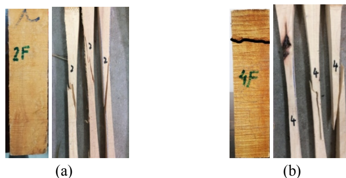
Fig. 3: Failure pattern under compression and tension for Ziziphus mauritiana (Bair) from city of (a) Khushab, (b) Jhelum.
