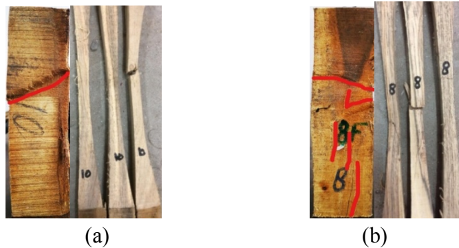
Fig. 6: Failure pattern under compression for Vachllia nilotica (Kikar) from city of (a) Dera Ismail Khan, (b) Khushab.
