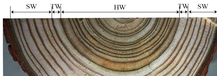
Fig. 2: The colors on samples distinguish of sapwood (SW), transition wood (TW) and heartwood (HW).
