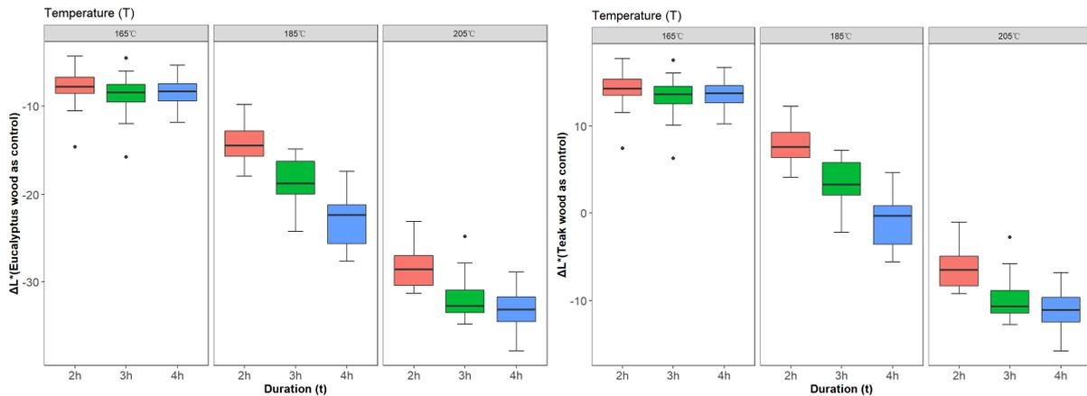
Fig. 1: Effect of heat-treated conditions on the lightness ( $L^*$ ) of eucalyptus wood.
