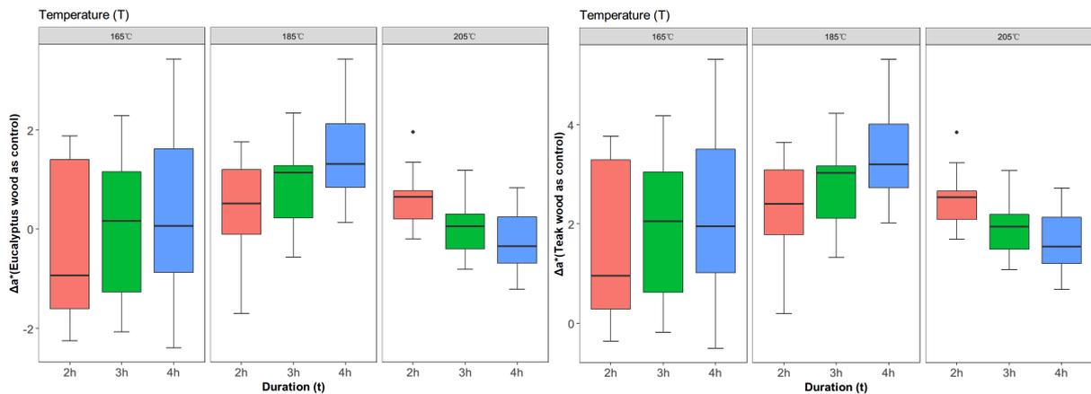
Fig. 2: Effect of heat-treated conditions on the red-green index ( $a^*$ ) of eucalyptus wood.
