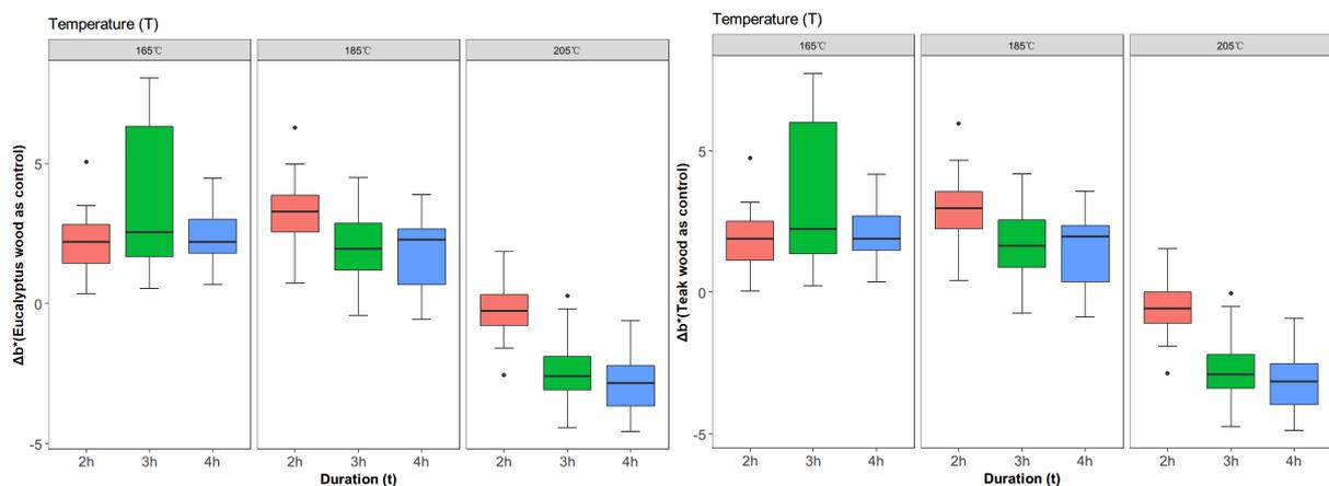
Fig. 3: Effect of heat-treated conditions on the yellow-blue index ( $b^*$ ) of eucalyptus wood.
