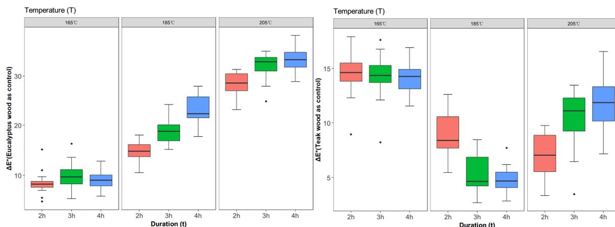
Fig. 4: Effect of heat-treated conditions on the total color difference ( $\Delta E^*$ ) of eucalyptus wood.
