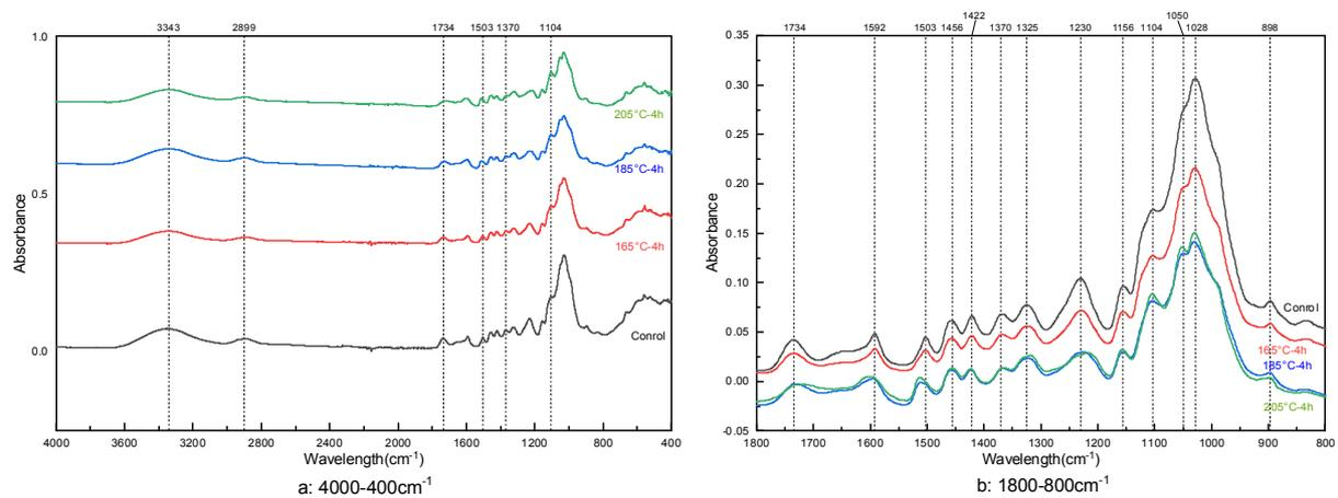
Fig. 5: IR spectra of untreated and treated eucalyptus wood at 165°C, 185°C, 205°C for 4 hours (a: 4000-400 $\text{cm}^{-1}$ , b: 1800-800 $\text{cm}^{-1}$ ).
