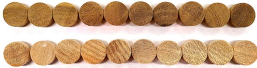
Fig. 1: Sample preparation (top line: heartwood, bottom: sapwood).
