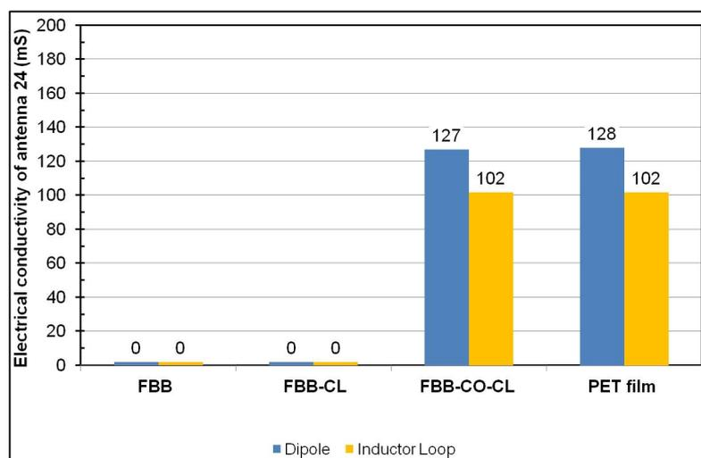
Fig. 5: Comparison of the dipole and the inductor loop electrical conductivity of the aluminium UHF RFID antenna 24 printed on commercial (FBB), calendered (FBB-CL), coated and calendered (FBB-CO-CL) paperboard and PET film.
