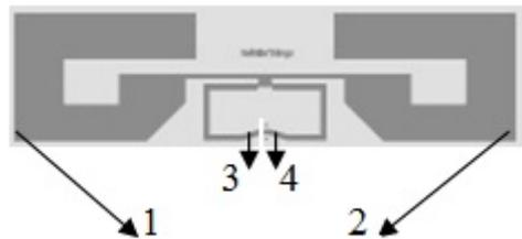
*Fig. 2: Measurement of the electrical resistance of the dipole (points 1 and 2) and the inductor loop (points 3 and 4) of the UHF RFID antenna 24.*
