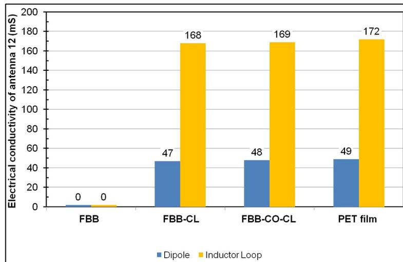
Fig. 4: Effect of plasma treatment (3 min) of commercial (FBB), calendered (FBB-CL), coated and calendered (FBB-CO-CL) paperboard and PET film on the electrical conductivity of the dipole and inductor loop of printed aluminium UHF RFID antenna 12.
