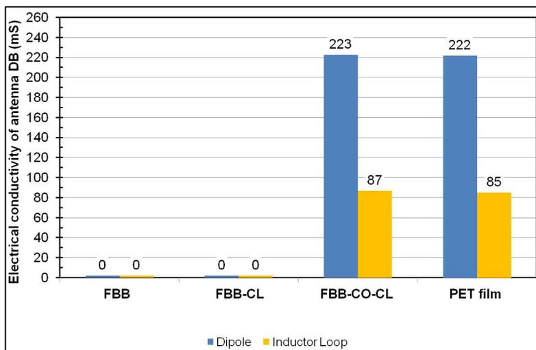
Fig. 7: Comparison of the dipole and the inductor loop electrical conductivity of the aluminium UHF RFID antenna DB printed on commercial (FBB), calendered (FBB-CL), coated and calendered (FBB-CO-CL) paperboard and PET film.
