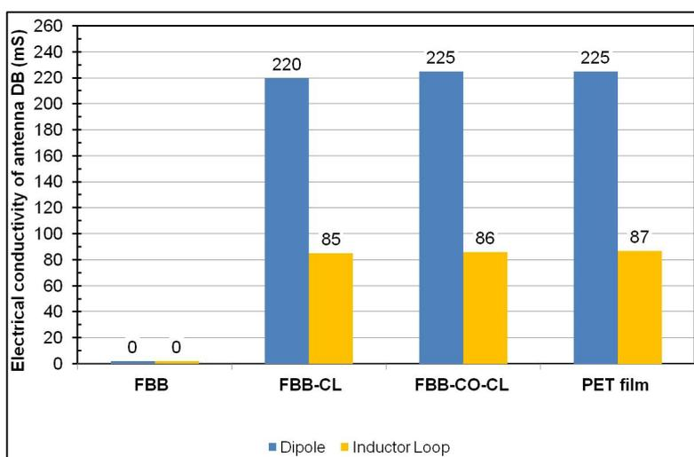
Fig. 8: Effect of plasma treatment (3 min) of commercial (FBB), calendered (FBB-CL), coated and calendered (FBB-CO-CL) paperboard and PET film on the electrical conductivity of the dipole and inductor loop of printed aluminium UHF RFID antenna DB.
