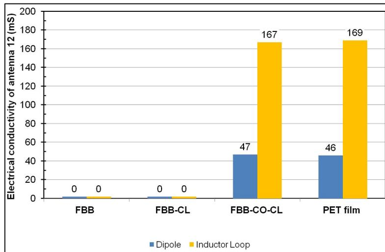
*Fig. 3: Comparison of the dipole and the inductor loop electrical conductivity of the aluminium UHF RFID antenna 12 printed on commercial (FBB), calendered (FBB-CL), coated and calendered (FBB-CO-CL) paperboard and PET film.*
