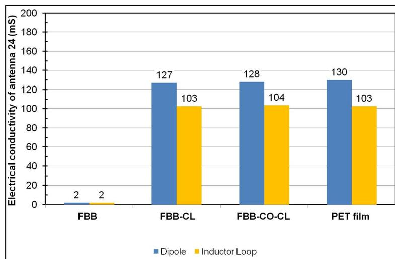
Fig. 6: Effect of plasma treatment (3 min) of commercial (FBB), calendered (FBB-CL), coated and calendered (FBB-CO-CL) paperboard and PET film on the electrical conductivity of the dipole and inductor loop of printed aluminium UHF RFID antenna 24.
