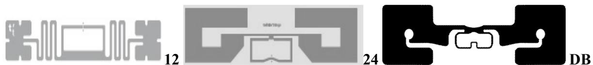
Fig. 1: Designs of symmetric UHF RFID antennas (not in scale).
