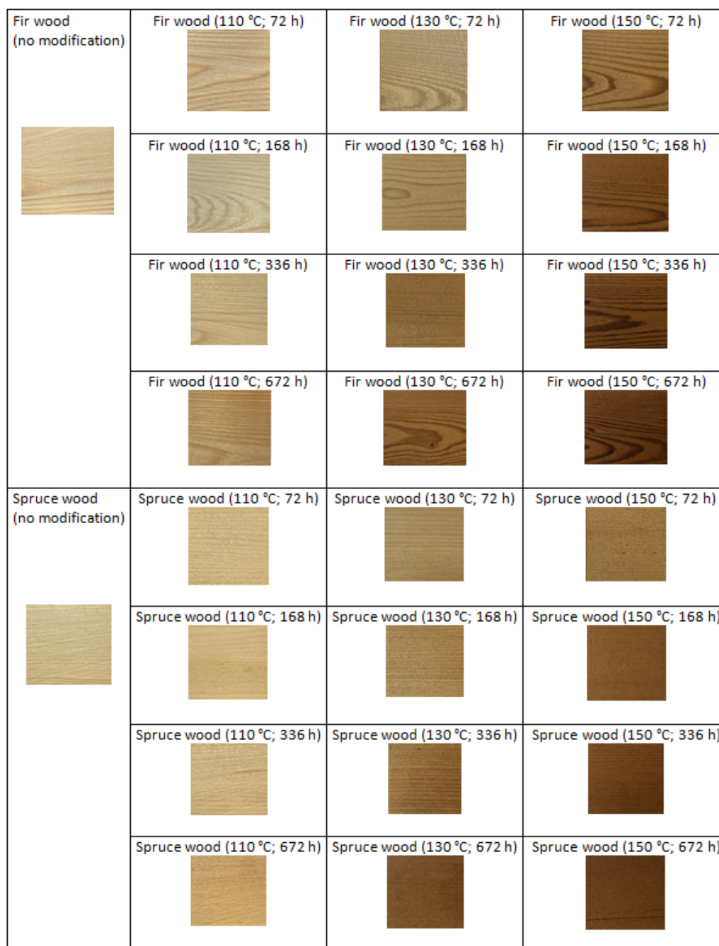
Fig. 2: Samples of fir and spruce woods before and after exposition by temperature in range from 110 to 150°C during 72 to 672 h.
