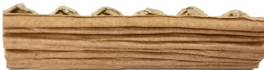
Fig. 6: Deformation mode of the linerboard.
