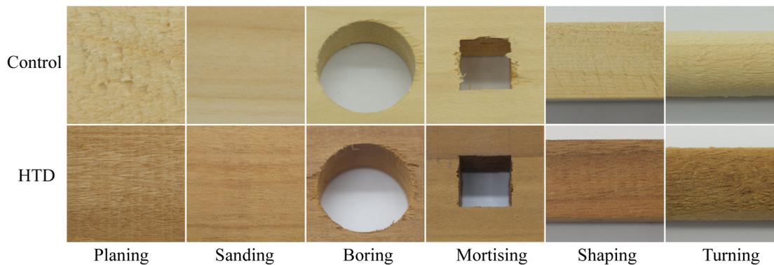
Fig. 5: Machining performance defect photos of the control and HTD.
