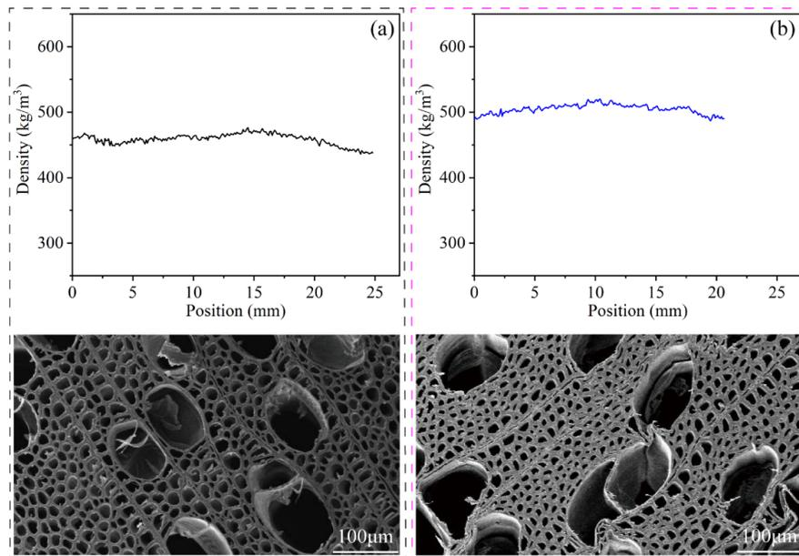
Fig. 3: Vertical density profile curves and SEM of the control (a) and HTD (b).
