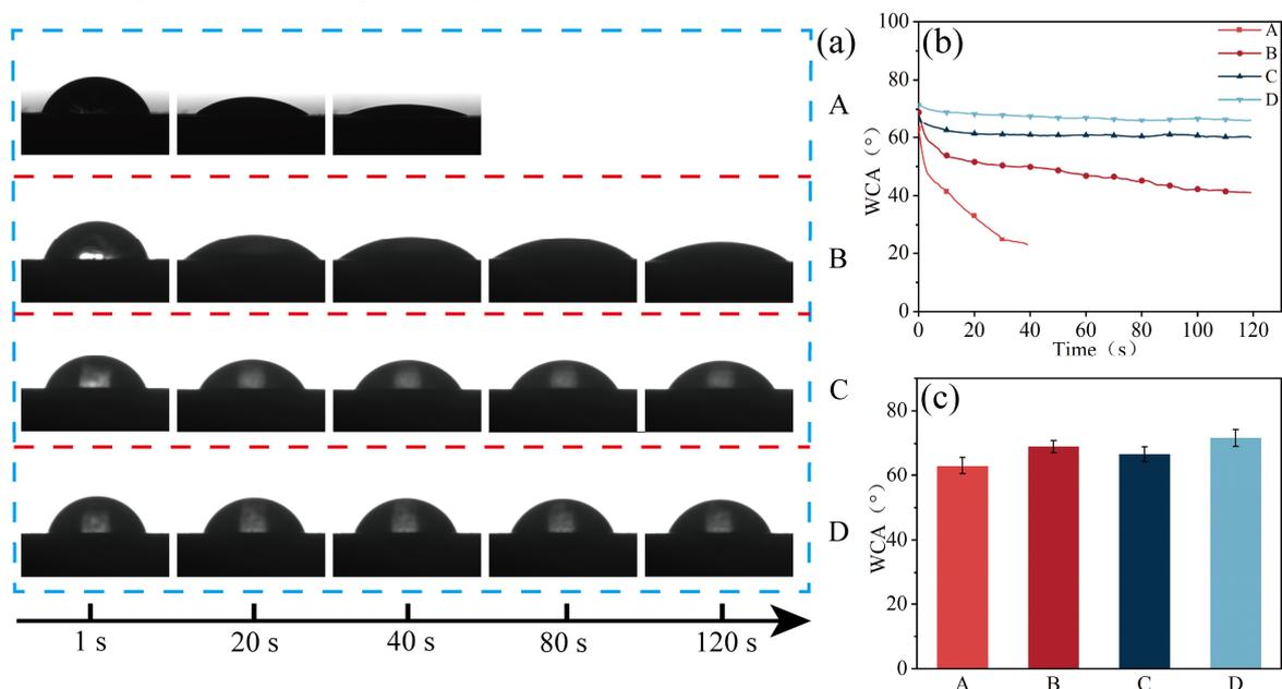
Fig. 8: Control and HTD's contact angles, (a) graphs of water droplets at different times of contact, (b) contact angle curves, (c) contact angle maxima; Where A and B are uncoated control and HTD respectively, and C and D are coated control and HTD.
