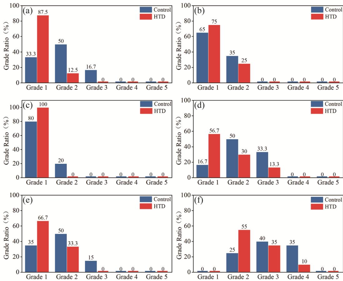
Fig. 4: Proportion of machining performance grade of the control and HTD: (a) planing performance; (b) sanding performance; (c) boring performance; (d) mortising performance; (e) shaping performance; (f) turning performance.
