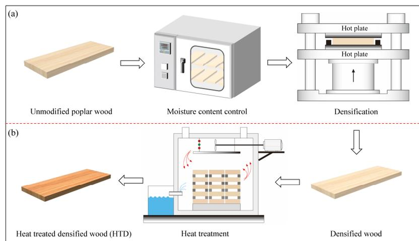
Fig. 1: Schematic diagram of densification (a) and heat treatment (b).
