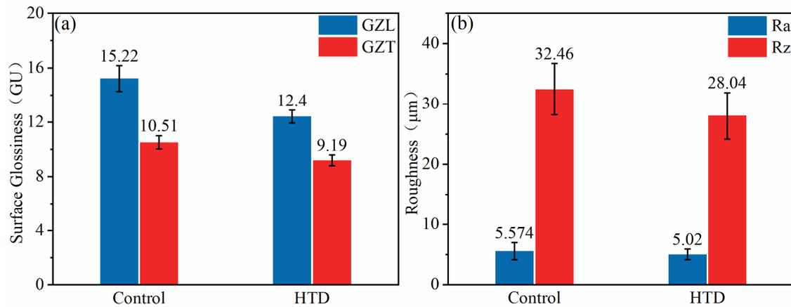
Fig. 6: Surface glossiness (a) and roughness(b) of the control and HTD after water-based UV paint coating.
