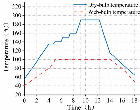
Fig. 2: Heat treatment procedure.
