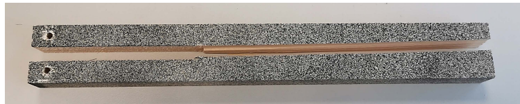
Fig. 6: Typical Mode I failure (crack opening) mechanism of tested specimens S1-S10.
